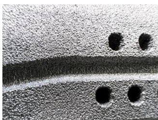
Surface Roughness of Metal 3D Printer Product
